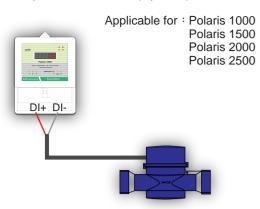
water meter with pulse output
