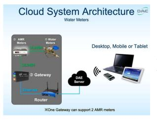
For monitoring up to 16 water meters remotely with cell phone, PC and generate billing report, you will just need **1 AMR KIT + 1 CC2030 KIT**.
