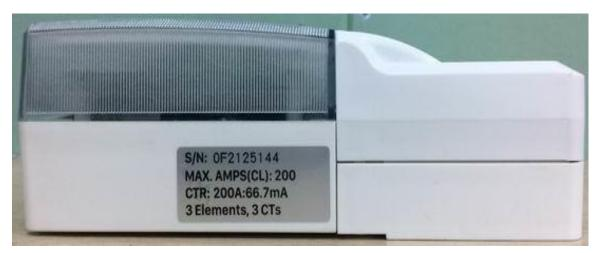
Side View of the Meter with Additional Identification Markings
