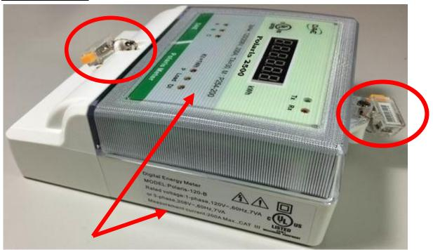
Side View of Meter with Front and Side Identification and Sealing Provisions
