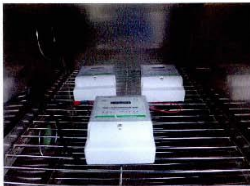
Figure 5 : Temperature and humidity test
