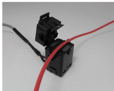
Step 2. Lay the load wire inside the opening
