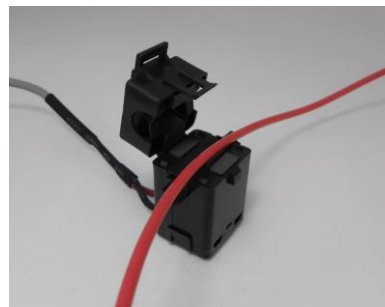
Step 2. Lay the load wire inside the opening
