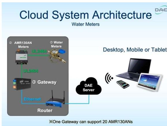
**1 DAE CC2030 KIT Gateway + 1 AMR130AN KIT** can read 1 water meter with pulse output (like DAE MJ-100n, PD-100, V-100P, VM-100P, and WP-200P) remotely with cell phone, PC and generate billing report. One CC2030 Gateway can monitor 20 meters (water, electricity, and gas).
